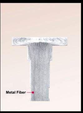
Manufacture part on a single machine using cold forming.
