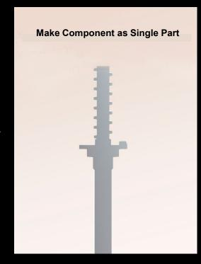
After assessing the final usage of the part with the customer, it was concluded that a single-piece cold formed part could be used in place of the original two-piece machined assembly.
