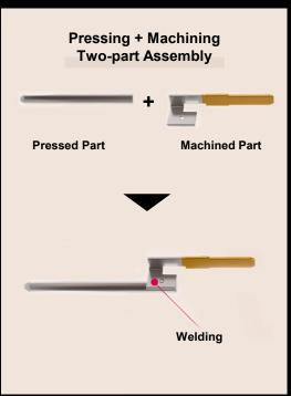
This part was originally designed as a welded two-part assembly, which led to lead-time and durability problems.
