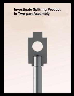
A study was conducted to see if this component can be split into a head part and a shaft part, which, when assembled, may provide the required concentricity more dependably than the original single-piece component.
