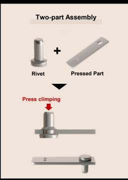
Two-piece assembly where a stamped plate and a cold formed shaft were fastened together (crimped).
