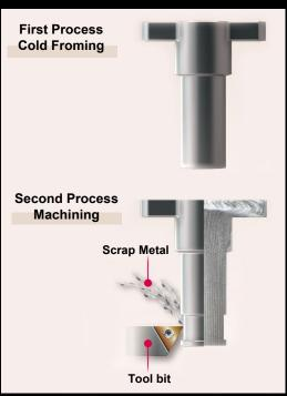
This part was originally manufactured in a two-step process, which led to increased scrap production and emissions.
